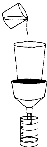
FIGURE 5. Test equipment for oil and water absorption.
